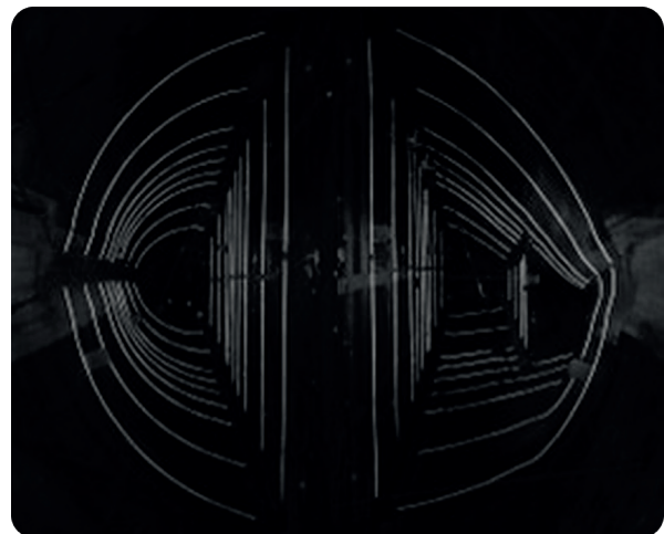
4. Illuminate markers and acquire footage as blade deforms
