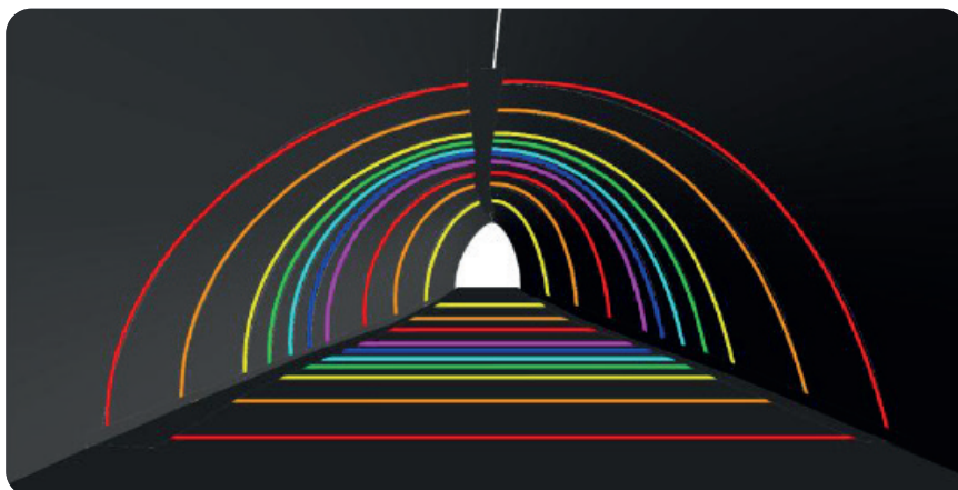
Figure 3 - CAD rendering of LE cavity to plan BODEM reflective marker positioning
