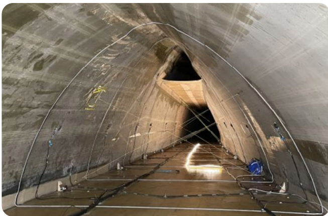
Figure 5 - internal view of the blade trailing edge cavity showing instrumentation
