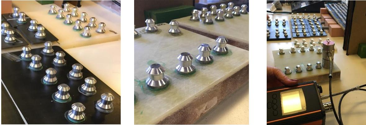
Figure 23 – Adhesion testing for different materials in connection with specified adhesive using SIKA DANMARK facilities in collaboration with DIS & Bladena
