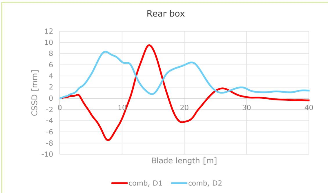
Figure 18: Cross-sectional Shear Distortion in the rear box
