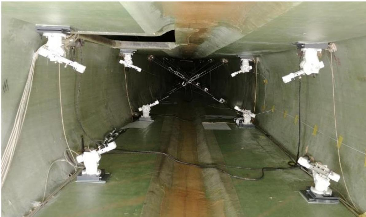
*Figure 73 - CSSDS test integration at DTU, installed FCMs inside the blade (left) and test rig (right)*
