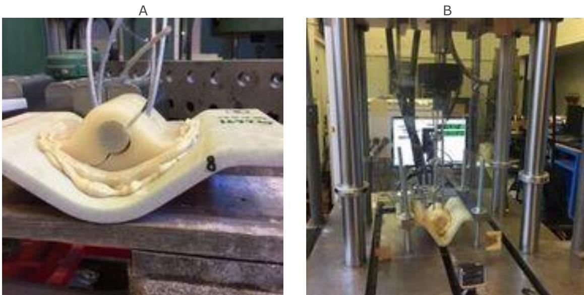
*Figure 83 - Test setup: A) details of bracket and corner mount and B) overall setup*
