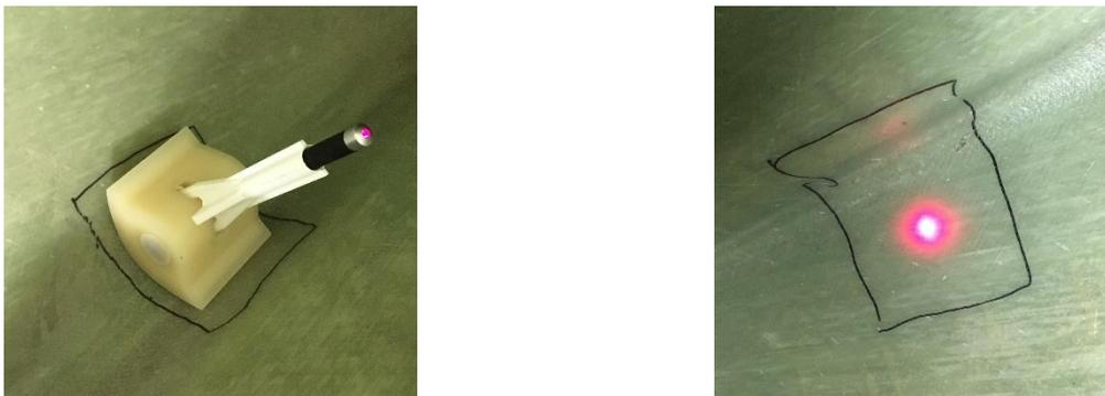
Figure 84 – Photo showing the specially made corner mount insert for laser alignment of brackets
