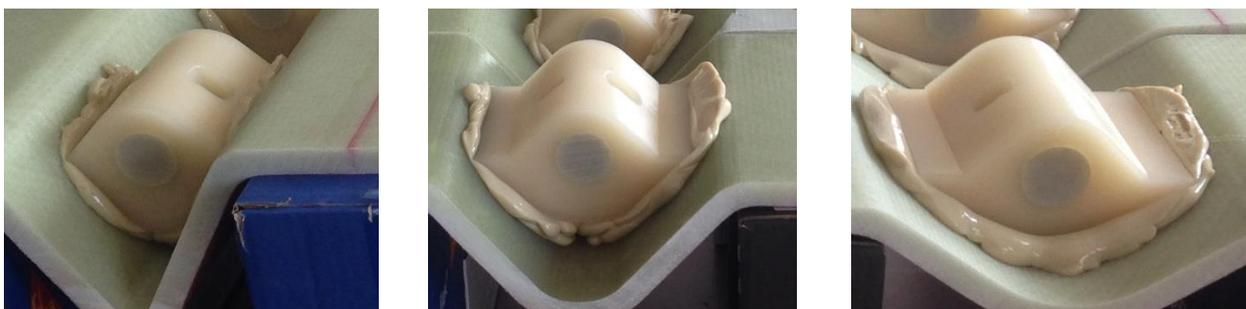
Figure 25 – Photo showing the 3 different corner mounts produced to cover angles between 60° & 140°
