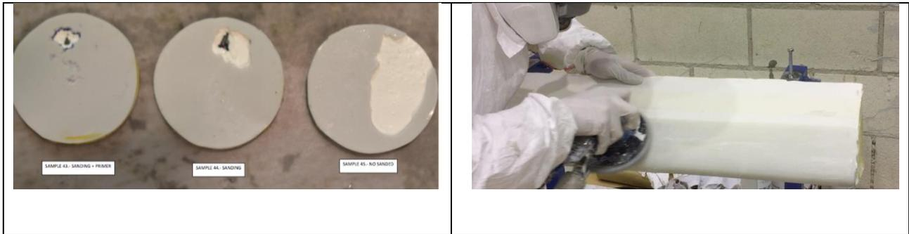
Figure 59 - (a) Rain erosion testing specimens. Erosion failure due to mass loss on surface and interface delamination for coupons depending on Primer application, Sanding and no sanding processing (b).
