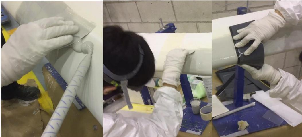
*Figure 50 - AHP LEP Service System application (Siemens Gamesa plant)*
