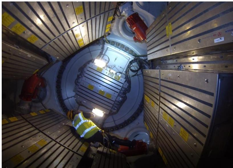
*Figure 89 – Technician inspecting cabling inside hub of LDT*
