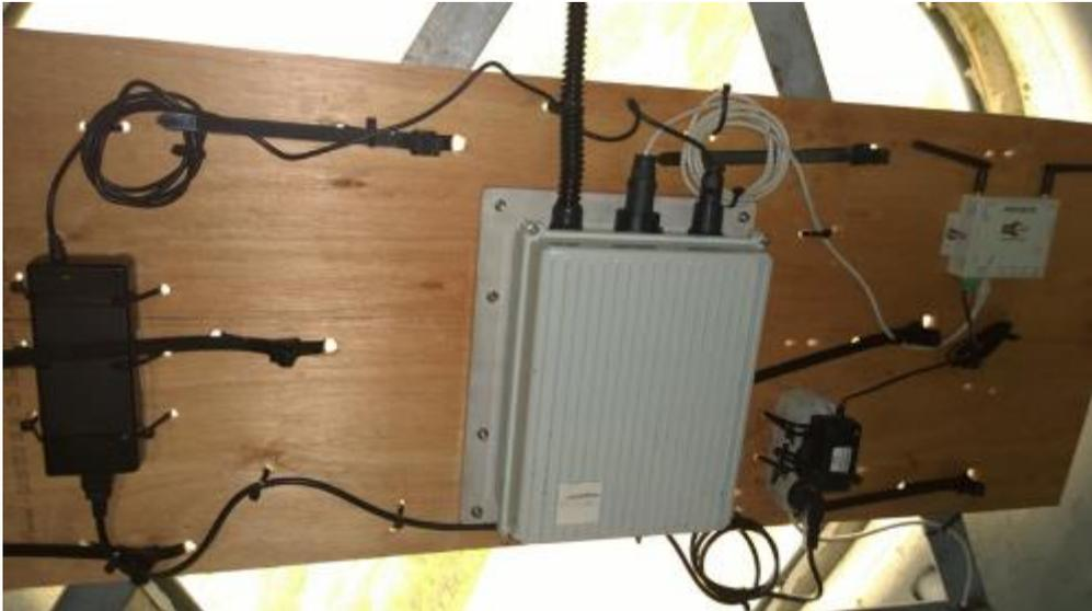
Figure 19: The WindMETER system mounted centrally in the hub with the power unit on the left, and data transmitter on the right.
