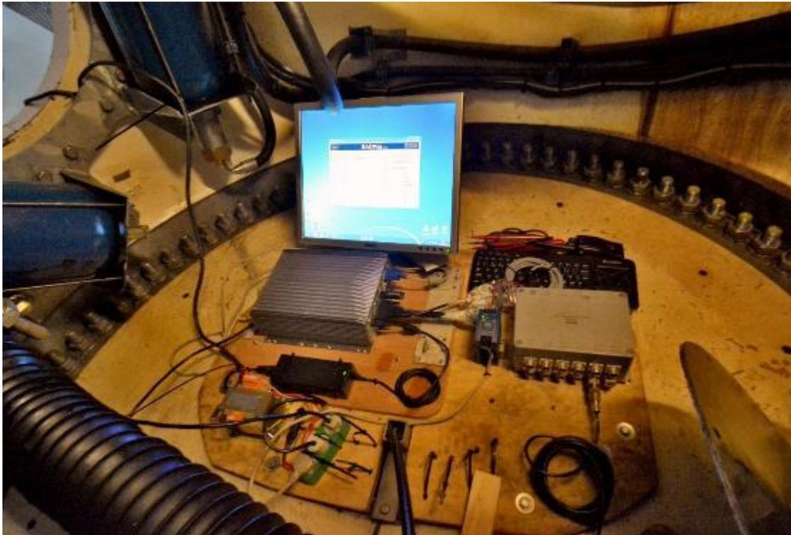
Figure 29. Data acquisition unit installed inside the hub.
