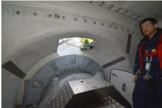
Figure 33. entrance hole to the hub from the nacelle.
