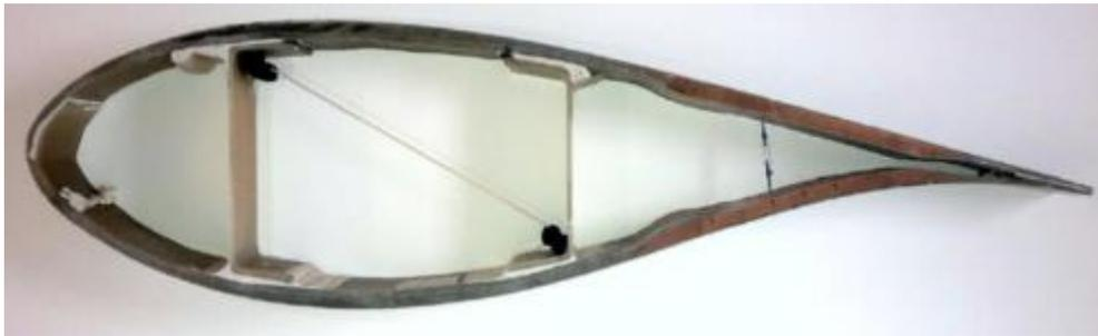
Figure 113: X-Stiffener implementation within blade structure.
