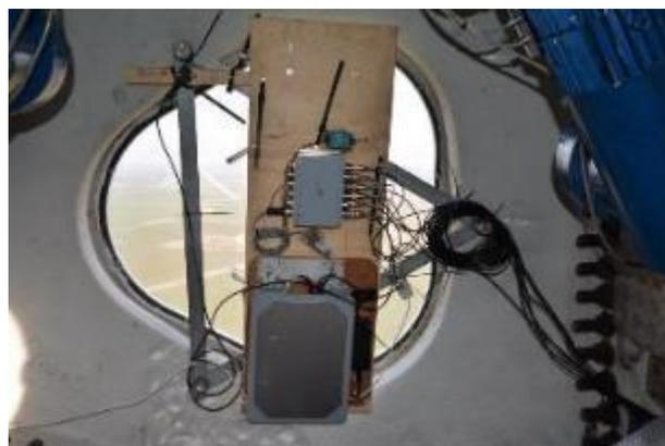
Figure 39. Data acquisition unit installed inside the hub.
