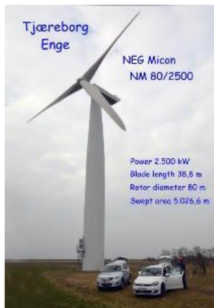
Figure 30. NM80 test turbine.
