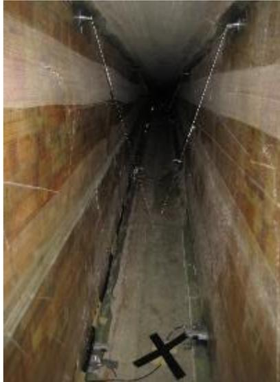
Figure 36. Inside of the blade mounted with measurement equipment.
