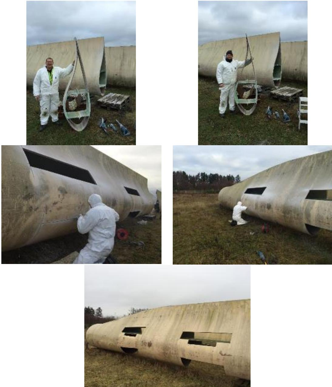
Figure 40. Cutting out of different blade specimens.
