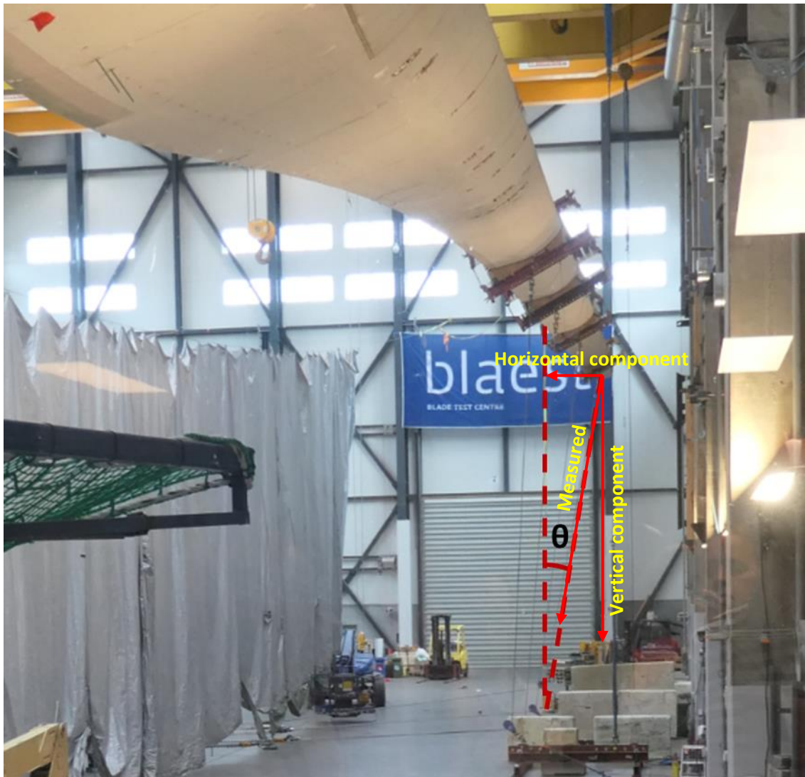
Figure 176: Blade deflection under loading
