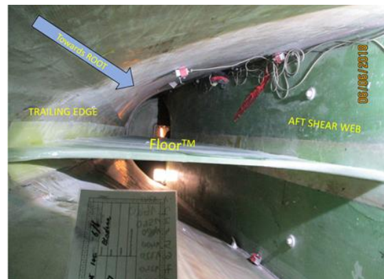
Figure 72: The Floor™ is designed to be retrofitted in the Root-transition zone of a wind turbine area between the aft shear web and the trailing edge. Here can be seen the first prototype of a Floor™ retrofitted in the LM58.7m blade.
