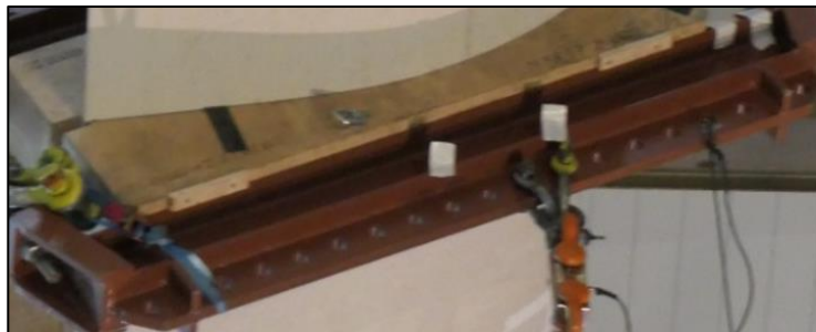
Figure 29: The same test was performed with and without and offset of the load application point towards trailing edge. In the figure is shown the wooden clamp at 49m from blade root with the two different load applications.
