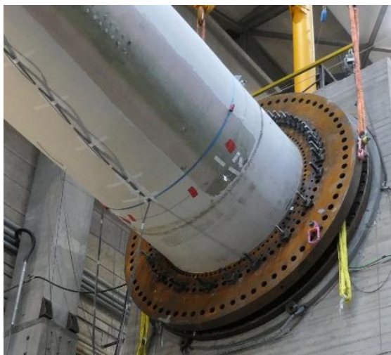
Subfigure 4a: Mounting of the blade
