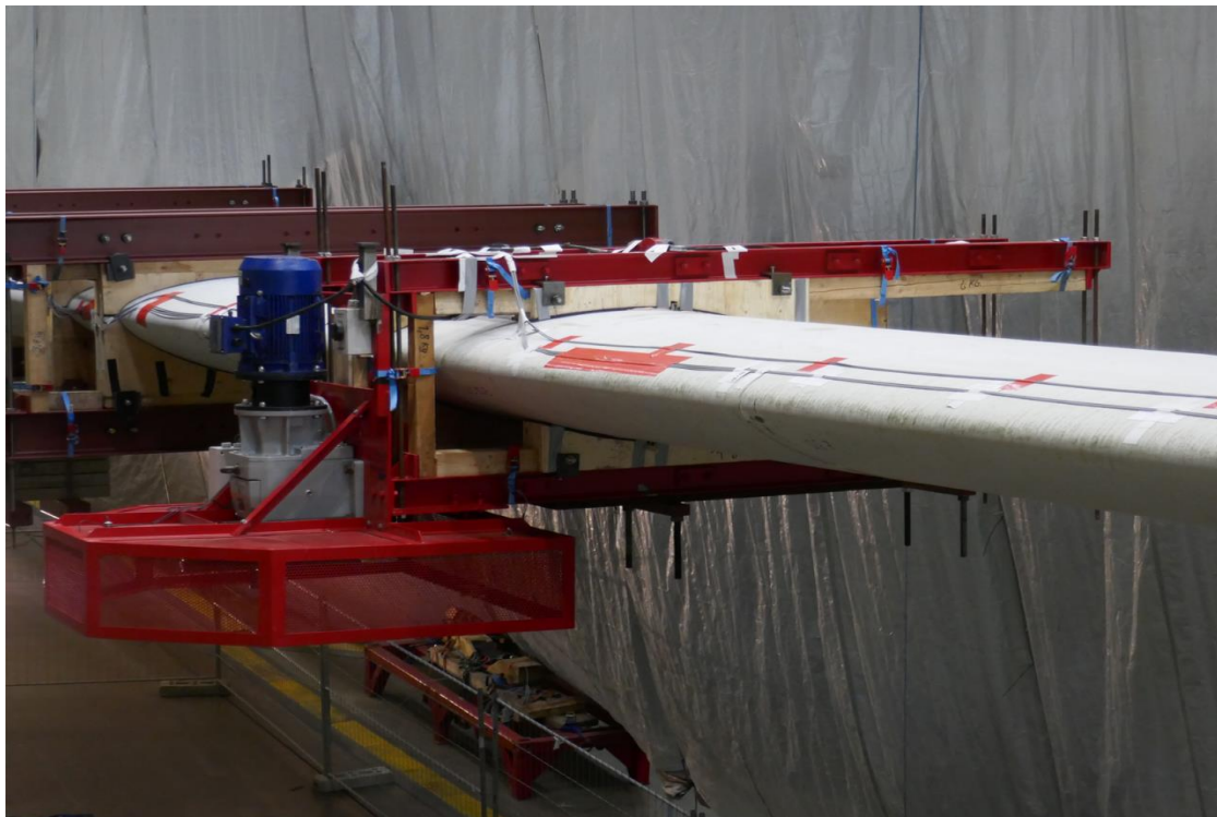
Figure 69: Full scale fatigue test. The clamps are mounted on the different sections of the blade to apply the appropriate load.
