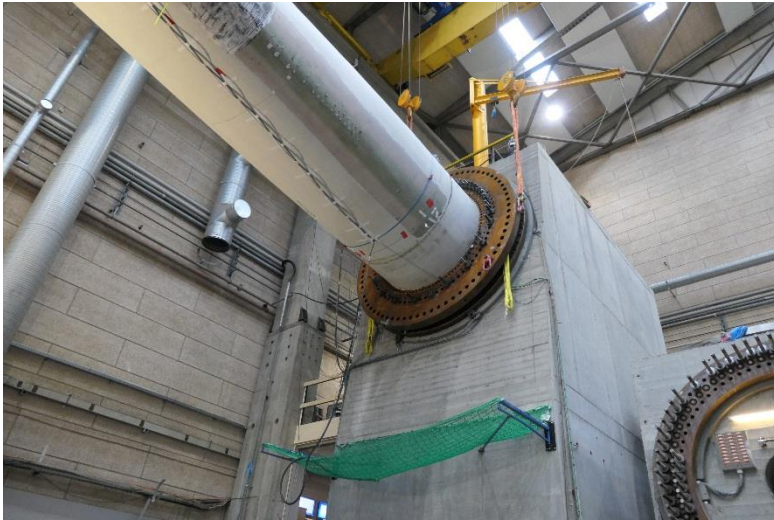
Figure 173: Blade root mounted on the test rig
