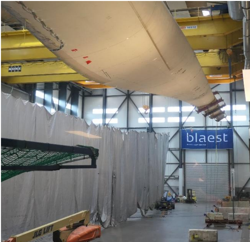
Figure 102: The LM58.7m blade is fixed at the root and hanging angled to ensure that the test pull towards the floor is in the right direction (combined load) according to the blade. Four clamps have been distributed in the outer 40% of the blade to apply the load.
