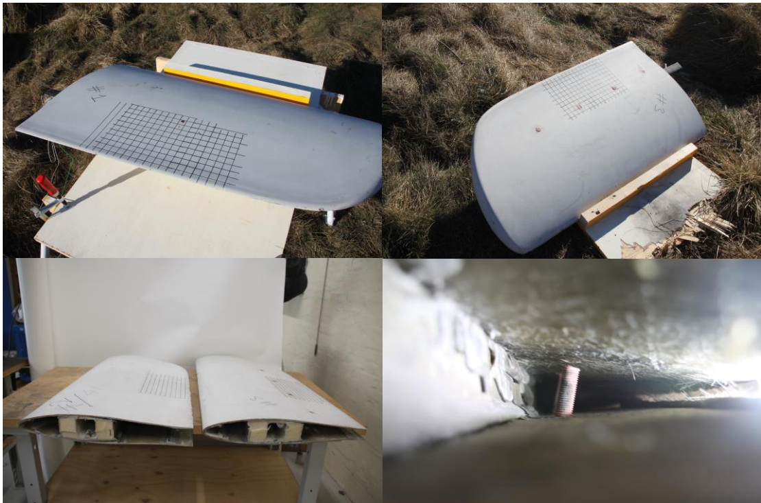
Figure 58: Test Specimens utilized for testing. All specimens were of length 1 meter. Two specimens without the struts were tested and one with the struts.
