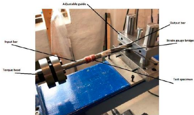
Figure 2-5 – Low strain rate torsional test unit
