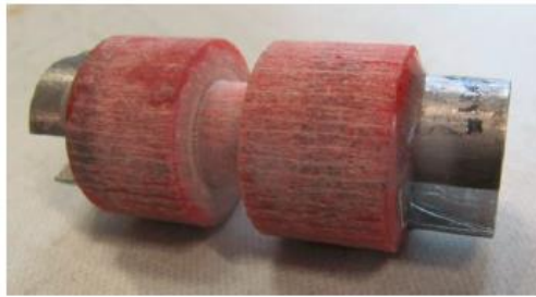
Figure 4.10 - Typical tests sample bonded to titanium end caps
