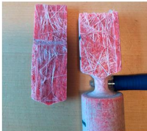
Figure 2-6 - EPR S1 30mm rod cross section, the white lines are the chopped glass fibres within the material.
