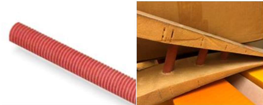
Figure 6: Strut solution for tip opening issue.
