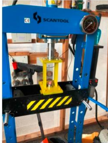
Figure 2-3 – Test sample mounted in hydraulic press
