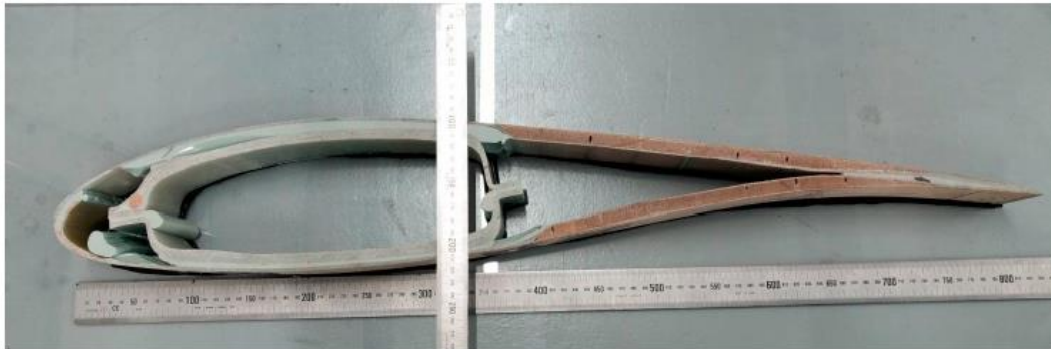
Figure 4.1 - Blade cross section 1 meter from tip
