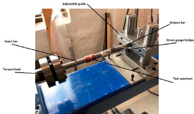
Figure 6.1 - The torsional split Hopkinson bar set up to carry out low strain rate testing
