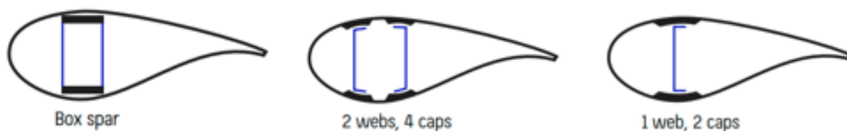
Figure 4 - Cross sections for different structural designs
